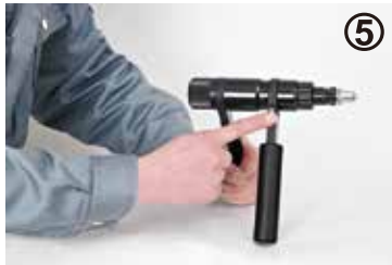
After setting, turn switch up, ready for releasing the nut
