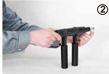
Adjust to ensure that all threads are meshed, and the front end of the threaded rod is slightly protruding, and the rivet nut is stick to the front side.
