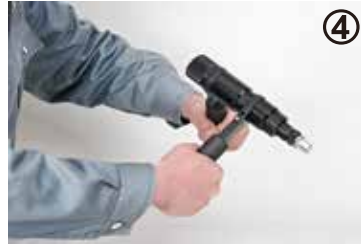
Move the handle for setting nut
