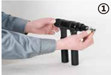
Put the nut on the mandrel, clockwise screw the nut on the mandrel
