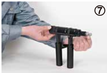
Counter clockwise turn the knob to release the nut
