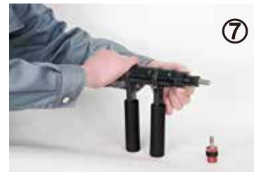
Clockwise turn the screw cover and mandrel for install onto the body
