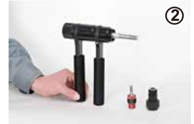
Unscrew the nosepiece from screw cover
